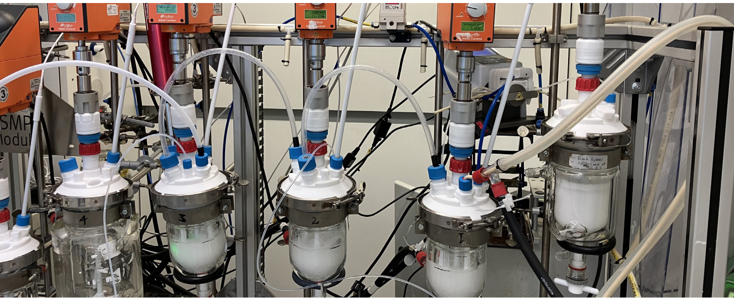
Image: Stage MSMPR setup with intermittent pressure driven transfer running Ibuprofen cryst.
